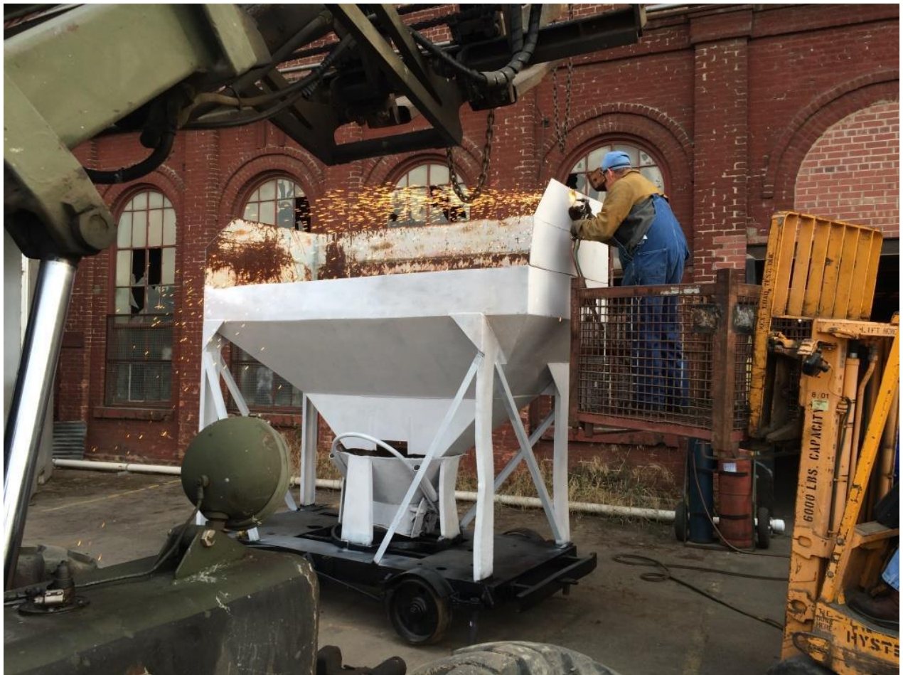
Cliff using his mighty torch to cut down walls of the new ballast hopper
