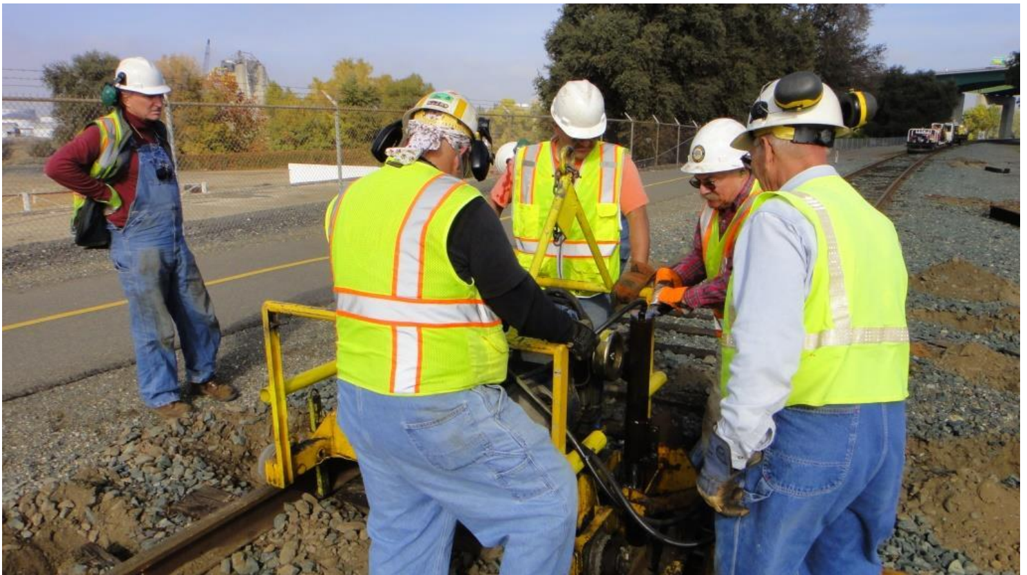
Mike H. fixes the faulty fitting on the lift-cylinder of the section-gang machine
