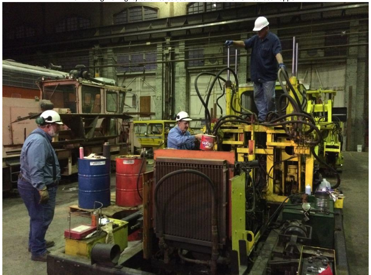
Frank W., Fred, and Scott start flushing the tir-shear's hydraulic system
